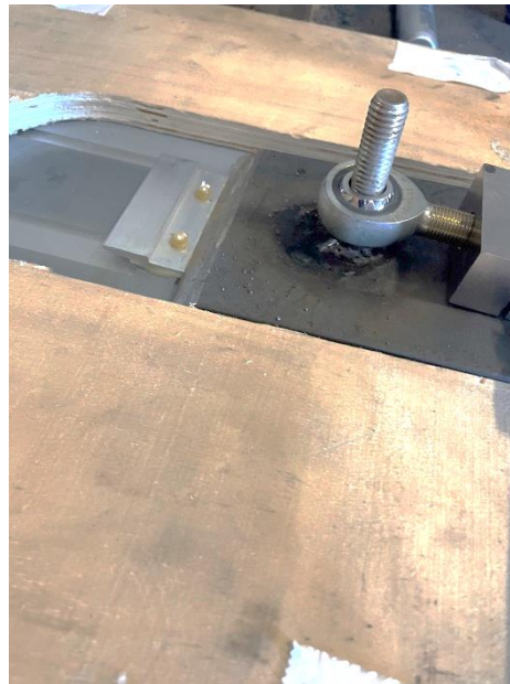
Photo No. 2 Jig Side View (clip and glass sample shown)
