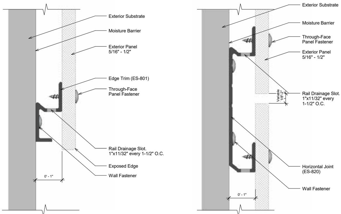
The ES-400 system is a typical exposed fastener system with the unique ability to be used either vertically or horizontally. WPS Exposed Fastener Panel is designed and engineered for commercial-industrial wall cladding panel that provides a traditional appearance. The ES-400 system is mechanically fastened with exposed fasteners and can be installed in a non-sequential pattern.
